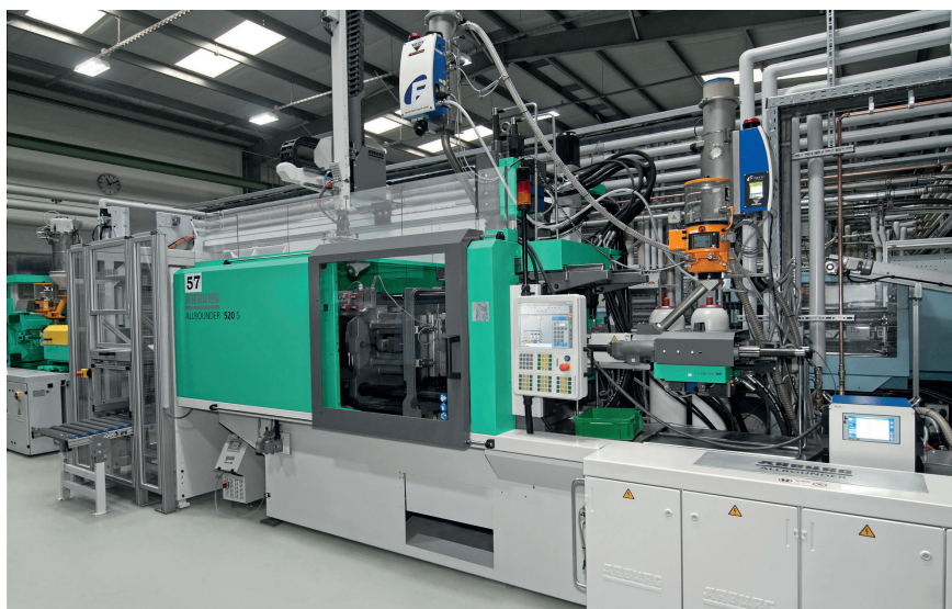
Fig. 3. Small, filigree cantilevers are produced on a two-component Allrounder 520 S injection molding machine using the assembly injection molding process. © Arburg
